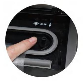
Make sure that the vacuum nozzle alignment is at the Make sure the vacuum nozzle alignment is at the Blow when you are at the blow function.
