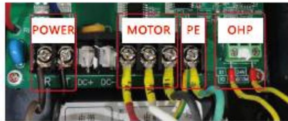
Single-phase Wiring (Actual Picture)
