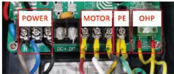
Three-phase Wiring (Actual Picture)
